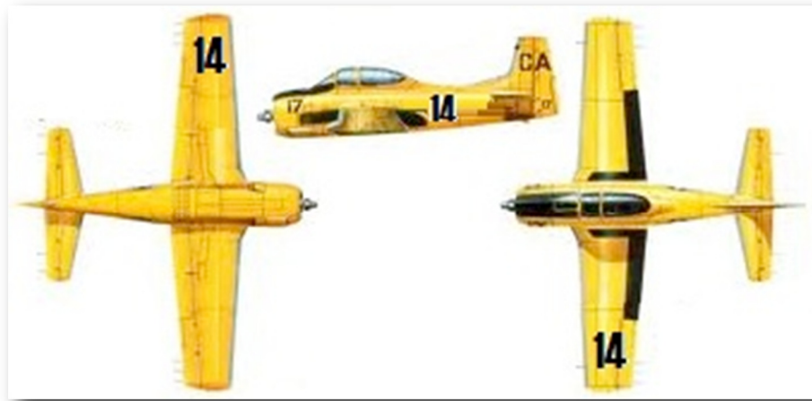
Figure 1: Illustration of how the race numbers should be applied to the wings and fuselage.
