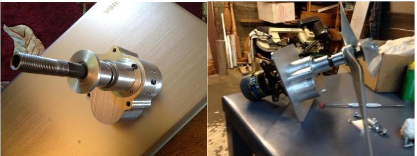
We decided to use an AXI 5345/16 for power. Ok now we need to test this monster. Earlier we had built a test stand to test motor and propeller combinations. We conducted many tests at progressively higher power settings. The first time we ran it, it started rolling down the driveway.
