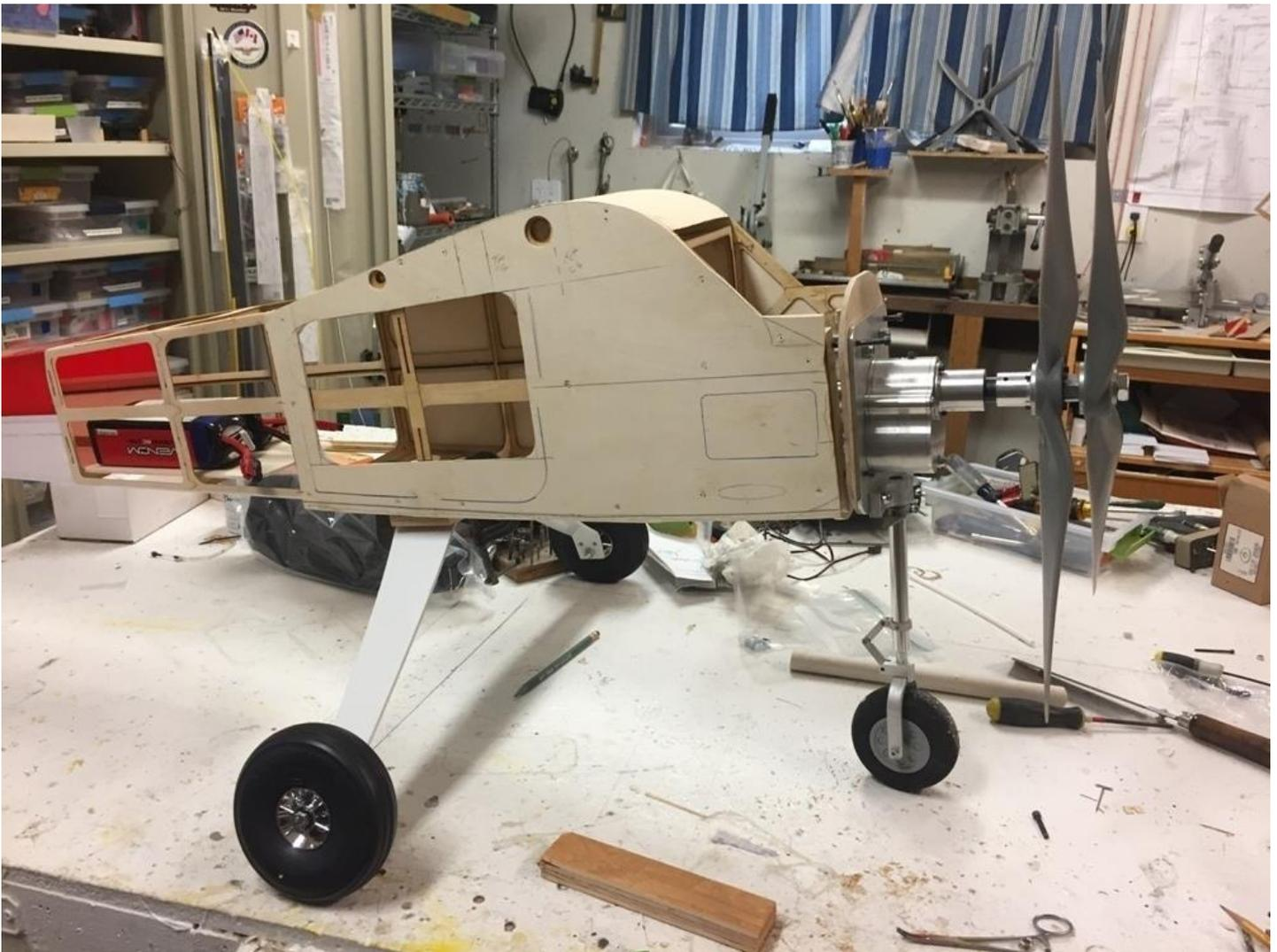
To change the angle of attack on the fuselage we ordered a new wider, taller and stronger aluminum main gear from TNT Landing Gear. The aircraft is now ready for flight test.
