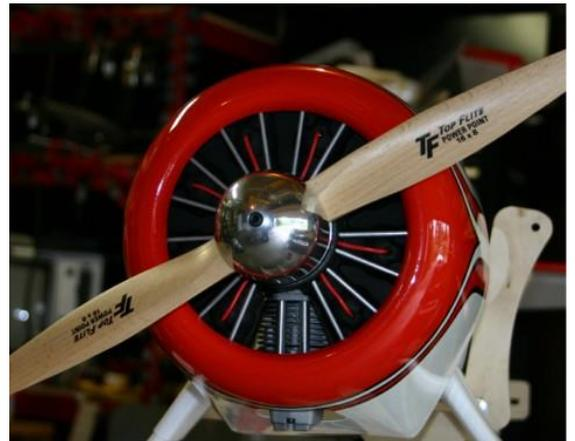
With the engine installed the only other thing necessary was to drill a couple of large holes, one through the inside back of the now, battery box and the firewall for the battery cables to exit and another through the firewall by the cylinder for the plug wire itself. As these were rather large to accommodate the large connectors, we then sealed them with some clear silicone.
