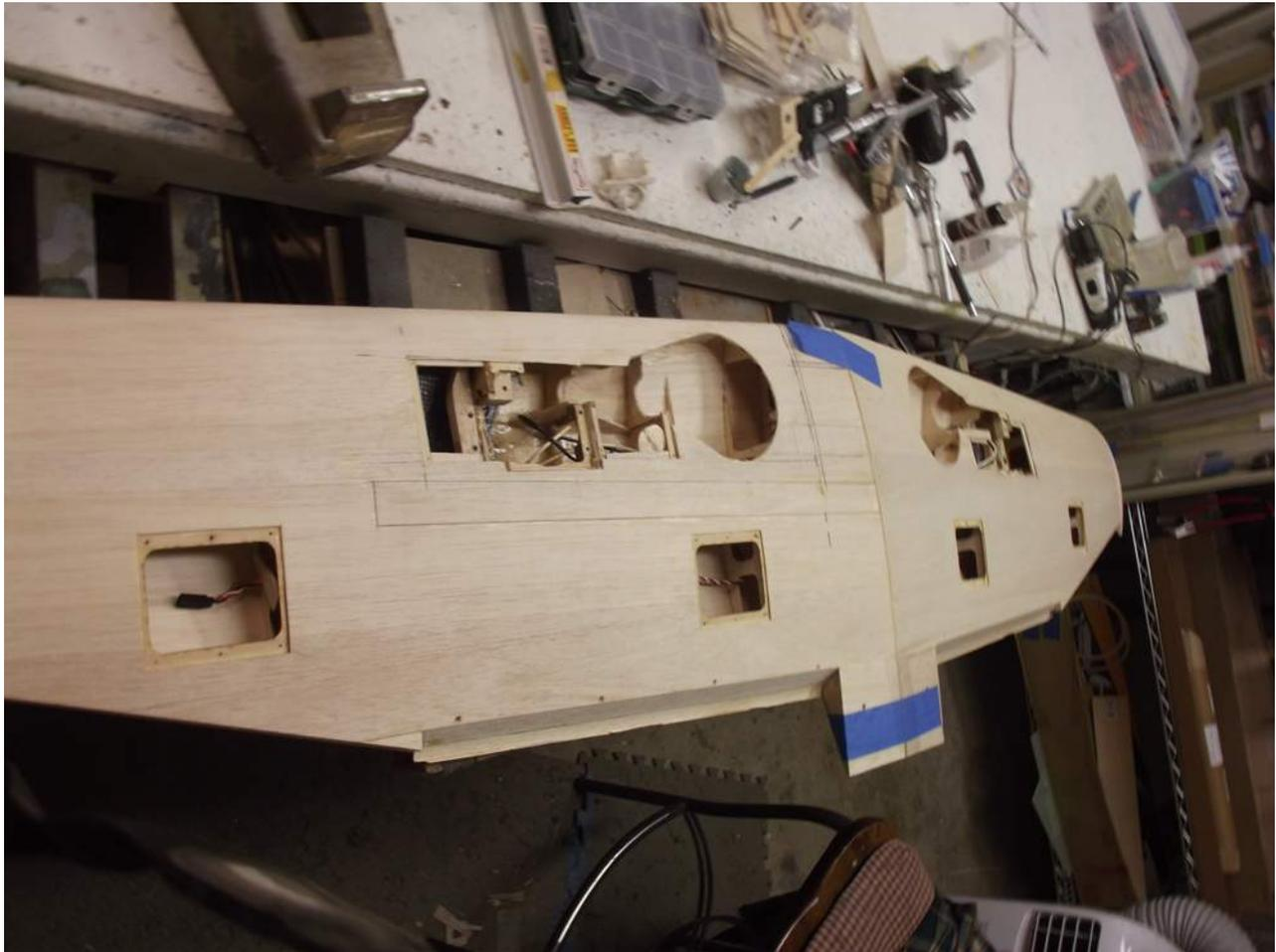
**When the epoxy had dried I sanded the bottom of the wing and applied a Carbon Fiber strip to the skin over the spar. Two coats of West System Epoxy was used to bond the Carbon Fiber.**
