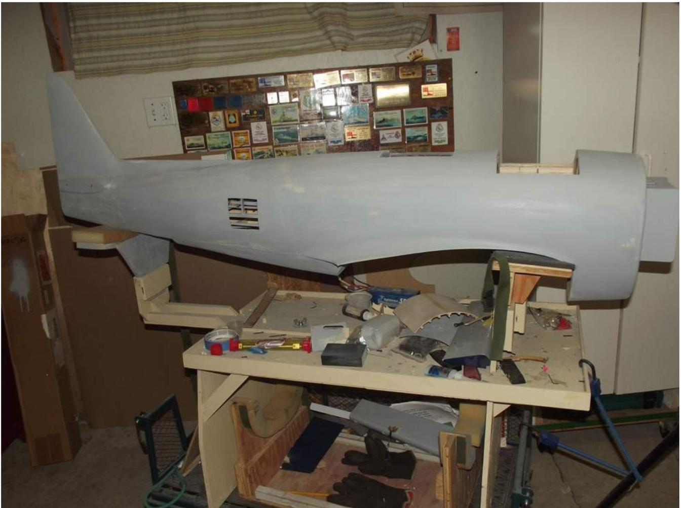
**Two heavy coats of primer were applied to fill the cloth weave. Most of which will be sanded away to a smooth finish.**
