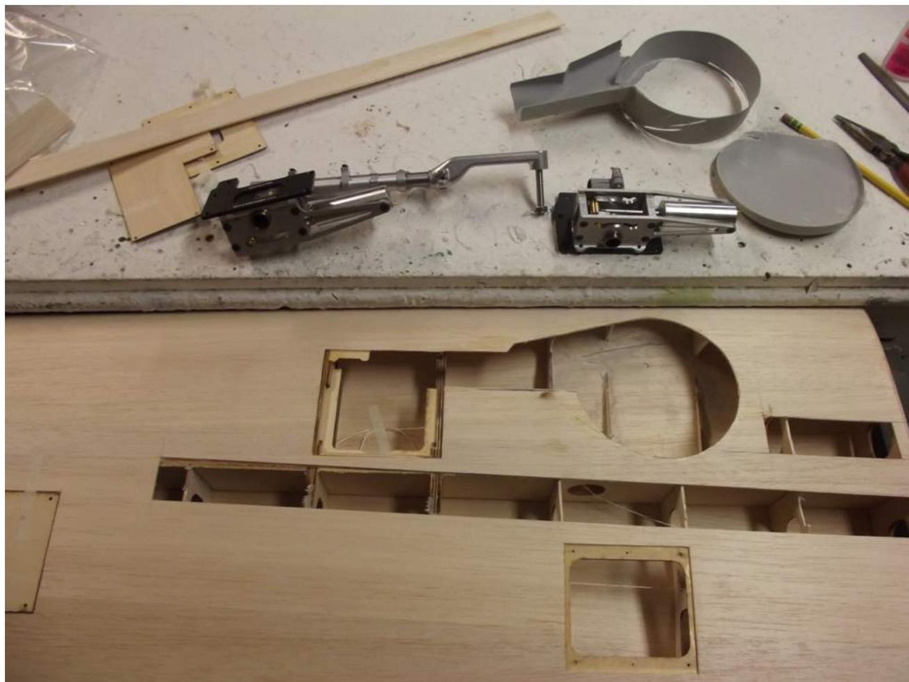
**The wing uses an aluminum joiner sandwiched between two light ply outer skins that slide about eight inches into the wing spar box on both sides of centerline. I think I will reinforce from centerline out one rib past the landing gear bay.**
