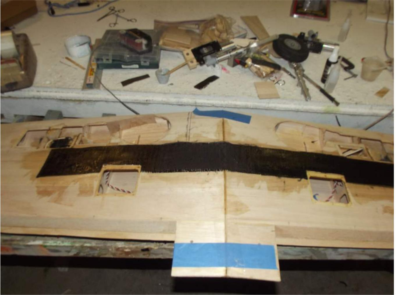
**Once the Carbon Fiber is sanded and smoothed into the wing I will cover the wing with  $\frac{3}{4}$  ounce fiber glass cloth. The shape of the wing is such the flat landing gear doors that came in the kit won't contour to the wing shape so it will be necessary to lay up fiber glass main and secondary gear doors.**
