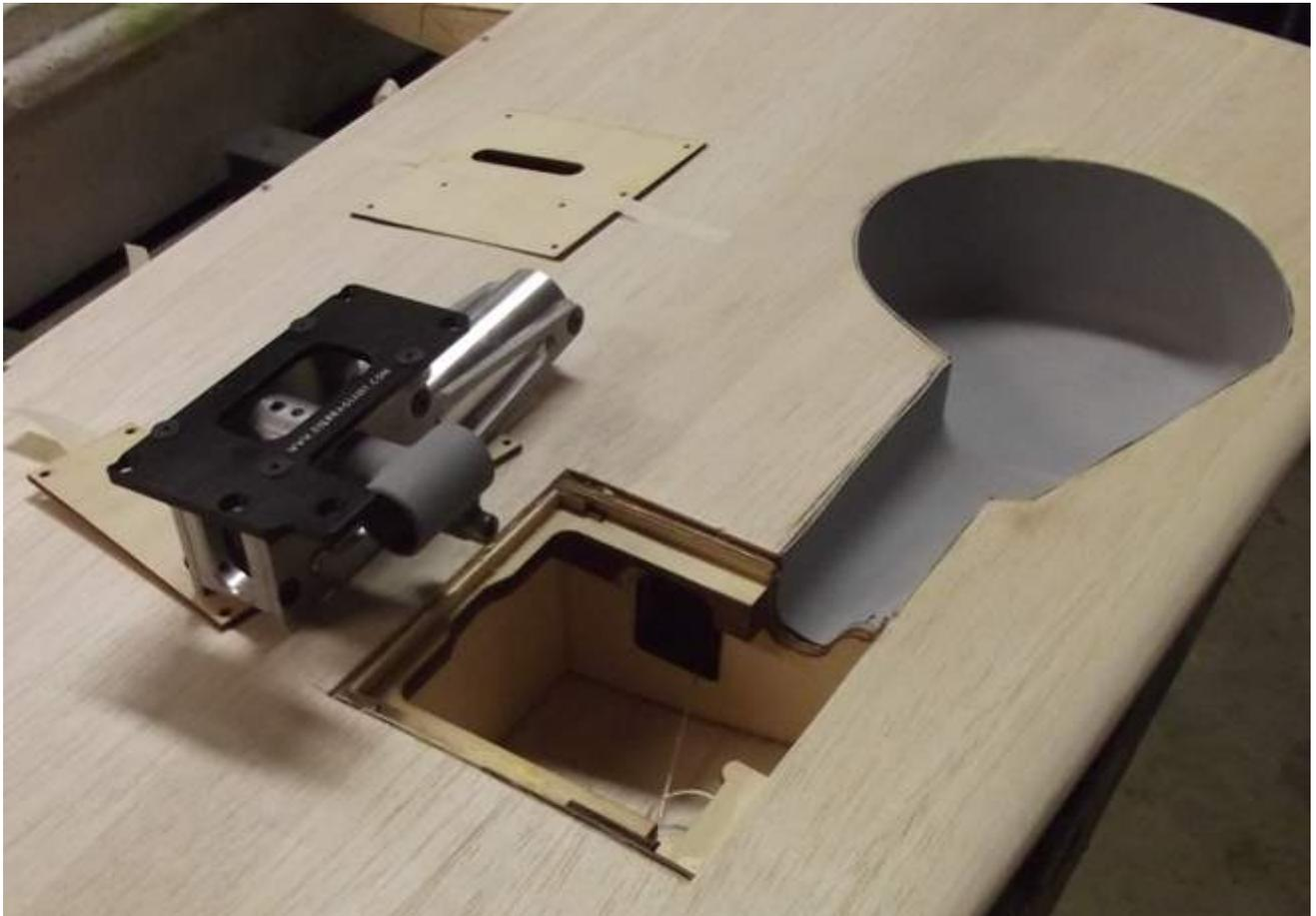
I also found a discussion on the weak main wing spar box. The problem seems to be the wing spar box is plywood that is not constructed out of heavy enough material. I have decided to strengthen the wing box with carbon fiber. I went to Dragon Plate Products [www.dragonplate.com](http://www.dragonplate.com). To see what is available.
