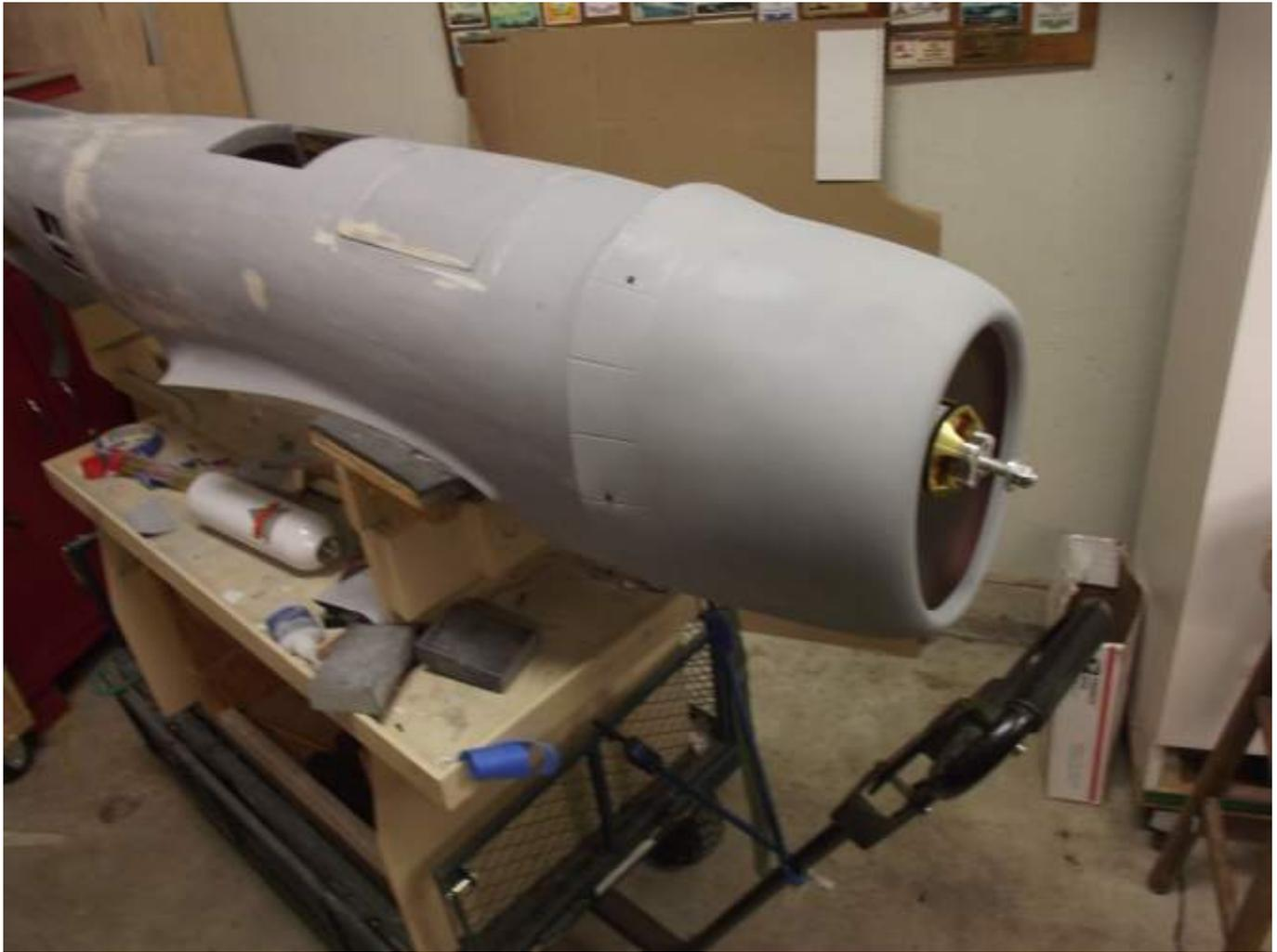
**The cowling is very lightly constructed. I will add a couple of layers of 3 oz glass cloth and epoxy to stiffen it up. Reinforcing the cowling is really necessary since I will be flying off some rough grass strips and ending up on it's nose is a good possibility.**
