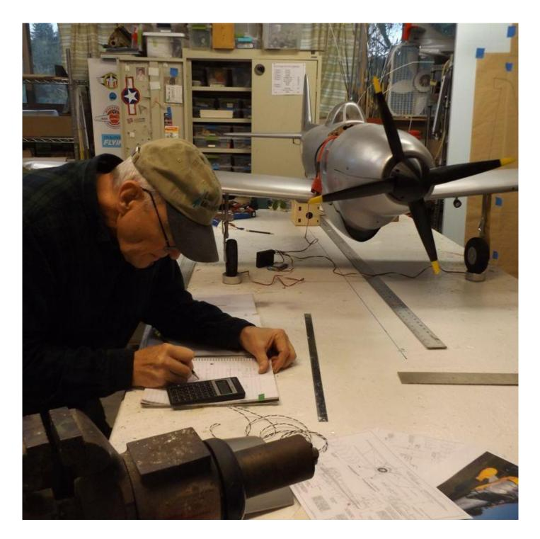
A few days before the aircraft was balanced using a mechanical balancer I have built on the end of my bench. We were just wondering how close we were to the correct CG before we added the paint. It was surprising how close we were. I have no doubt this plane would have flown with no further balance refinements.
