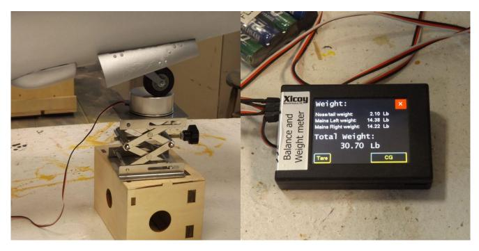
Drawn on the bench we have the aircraft centerline, the location of each of the wheels on the scales and the nose of the aircraft relative to zero is entered.
