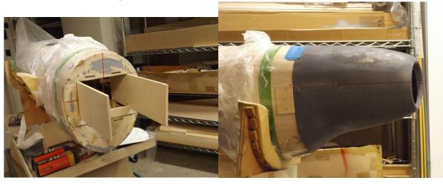
Next we positioned the gearbox and installed the foundation mounts for the cowlings.
