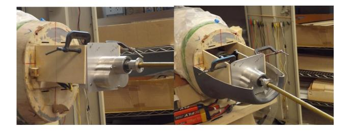
We used a 15 inch brass tube over the propeller shaft to verify the thrust line was exactly on aircraft centerline. Then we bolted the full powertrain into the fuselage.
