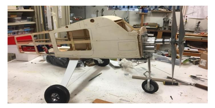
Republic extended the nose of their P-47 to compensate for the length of their gearbox and the larger motor. The R3350 that replaced the R2800 was about twice its length. This required a longer and slightly rounder cowling. We decided to use the lost foam casting pattern method. We scaled the cowling and plotted the cross section every two inches. We used adhesive spray to stick the printed plots to the foam. Next, we stacked them on a threaded rod through the center line.
