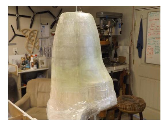
After the glass dried, we applied automotive glazing resin and sanded.
