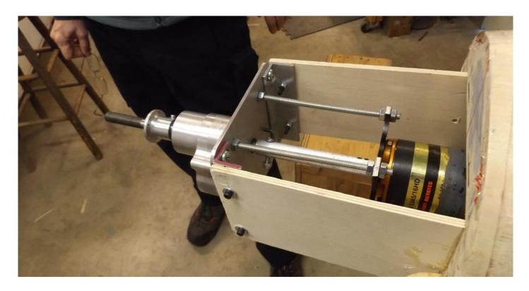
On our test plane the motor was just behind the firewall bolted to the gearbox. For weight and balance purposes we moved the motor six inches behind the gearbox.
