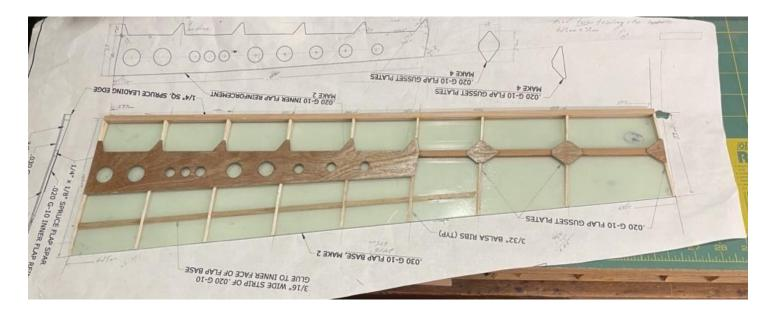
Both wings are now framed up on have the top sheeting installed. With little 4"x48" 3/23 balsa available several smaller sheets had to be edge bonded to produce a sheet of the necessary size. Bob has a large sheet of glass on one of his benches where he can cut and join balsa on a truly flat surface, what a good idea.
