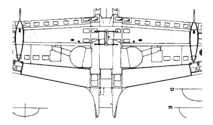
The basic problem is as the main gear retracts the wheels must move aft enough to clear the spar and rotate slightly to fit inside the thin wing.
