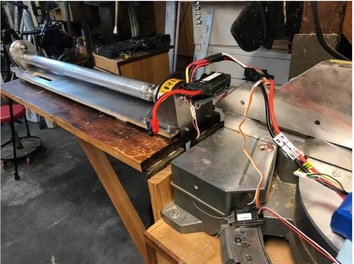
The first run was conducted using a 4s battery. Things went smoothly although the thrust bearing retainer nut on the gearbox loosened. We did notice a slight amount of wobble on the shaft coupling on the motor end. The drive tube is bonded to the shaft coupler we may have relook at that. Next, we will secure the Torque Plate to a test fixture and run it
