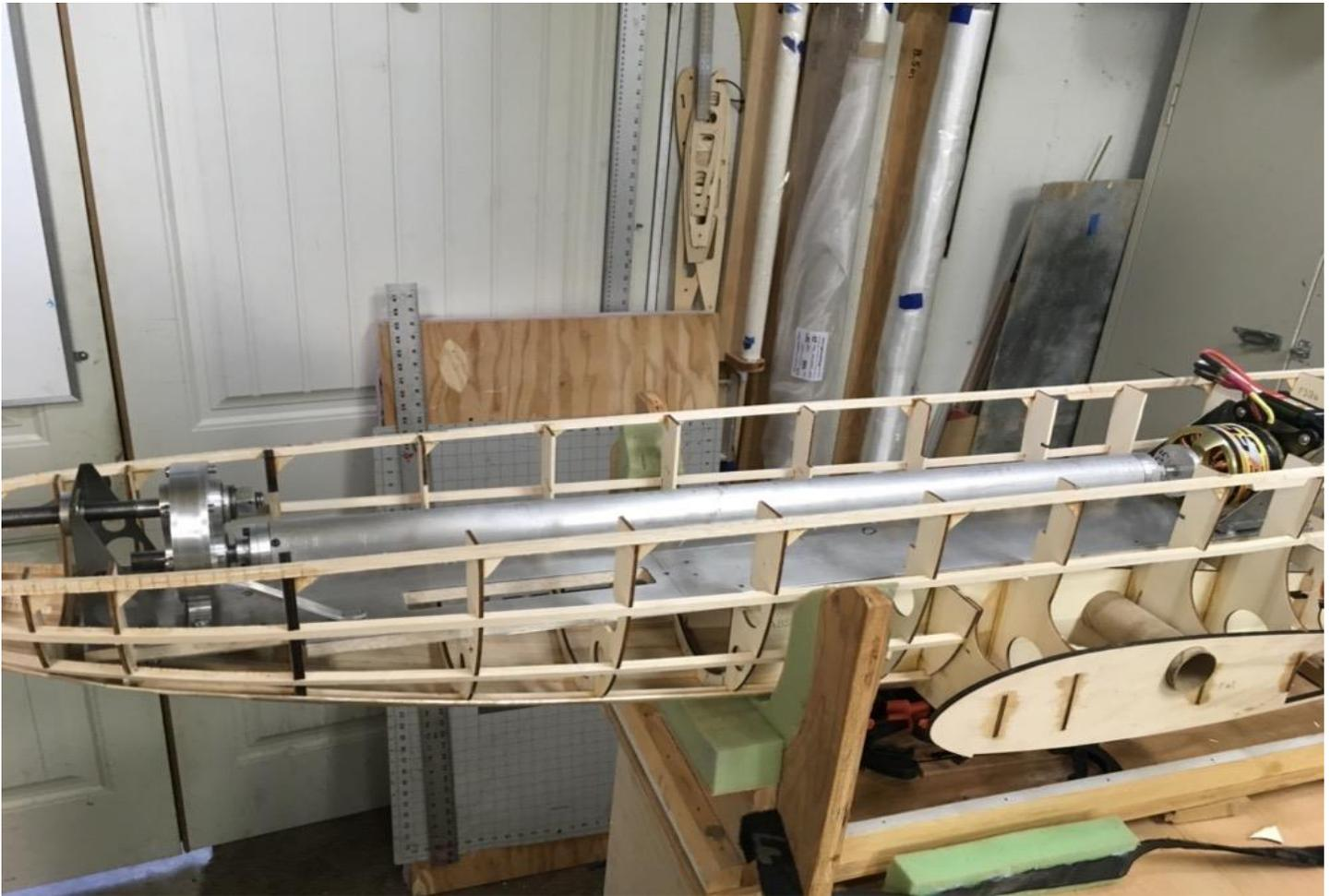
Next, we clamped the unit on the bench and ran it for a while on 6s. We recorded the watts and amps at 25% and 50% throttle. Everything seems fine so lets put a propeller on and do some low speed running.
