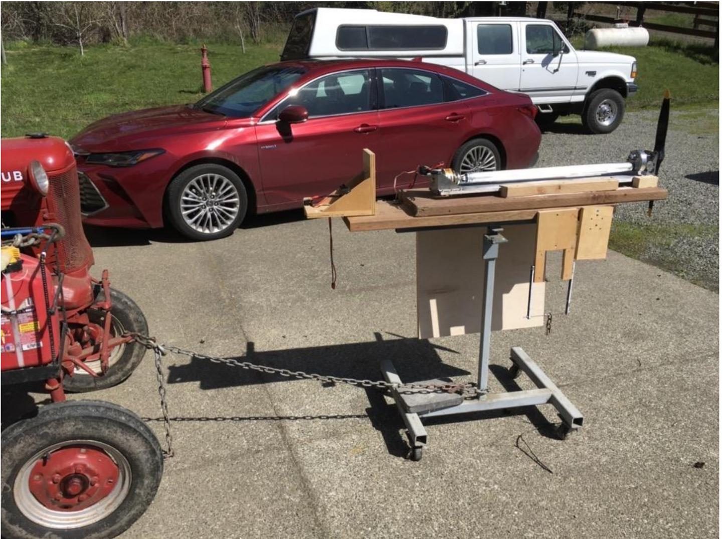
We never got past half throttle because we had one of the driveshaft tube screws kept coming loose. After about three minutes it would back out about half way. We couldn't tell if the Loctite failed, or did we forget to apply it. We don't know. We decided let's just go ahead and safety wire all the screws on the rotating parts and get on with the testing. We also decided to add a hard point below the ESC on the motor mount to allow us the attach the strain gauge to the motor centerline.
