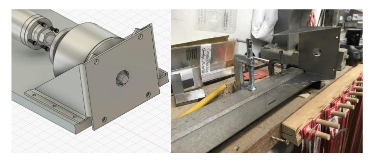
Our plan is to install the ESC on the back side of the motor mount. Doing this allows us to remove the complete propulsion system intact and go right into the test stand. Problems can be worked out away from the airframe.
