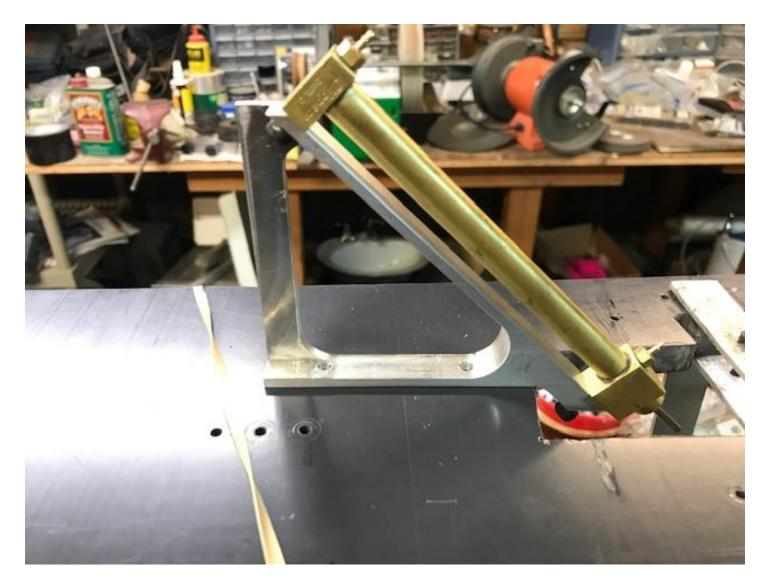
It was replaced by a shorter and stronger cylinder which again resulted in a linkage design change. Now all the ugly temporary linkage with all the holes drilled in them is being replaced.
