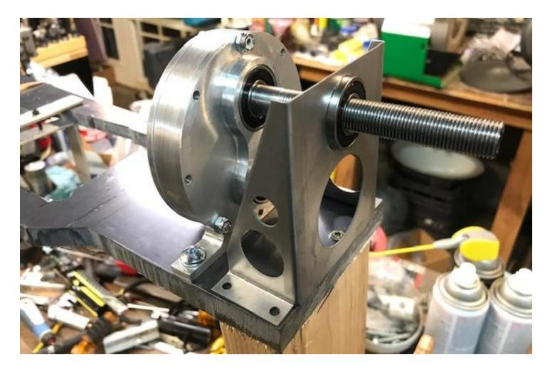
While waiting we finished the design of the nose gear. We had a couple of false starts on the actuator assembly. We first used a Clippard pneumatic cylinder thinking we needed about a four inch stroke. A problem was encountered was while folding the For Link and the Drag Link swing in two conflicting arcs and as they pass through the conflicting center point to over center lock something has to give. The Clippard cylinder was not strong enough to allow the passing.
