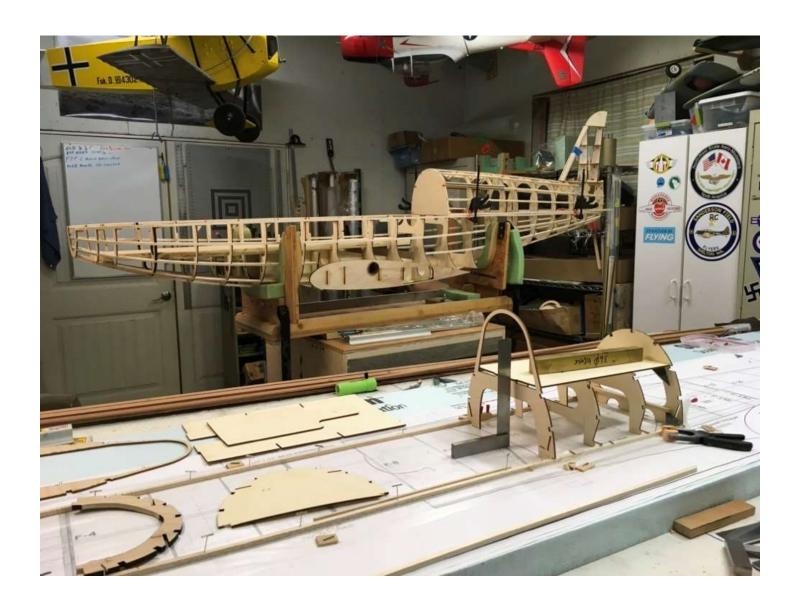
Building the airframe this way the propulsion system is easily removable. Any and all servicing or adjusting can be done on the bench. To stiffen things up a bit the removable section of the fuselage has a 1/4" hardwood stringer attached.
